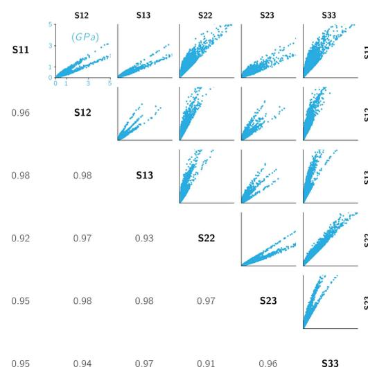
Fig. 8: The correlations of the first 6 orthotropic stiffness parameters of the decomposition size of 1.2 mm.
