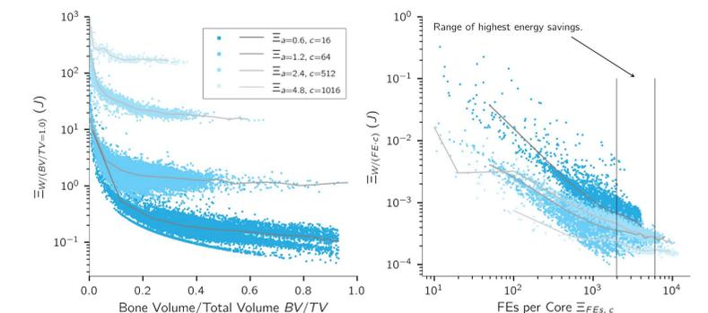
Fig. 9: Different serial and parallel parts of computing a single subvolume lead to a characteristic relationship between the Bone Volume/Total Volume (BV/TV) ratio and the energy usage.
